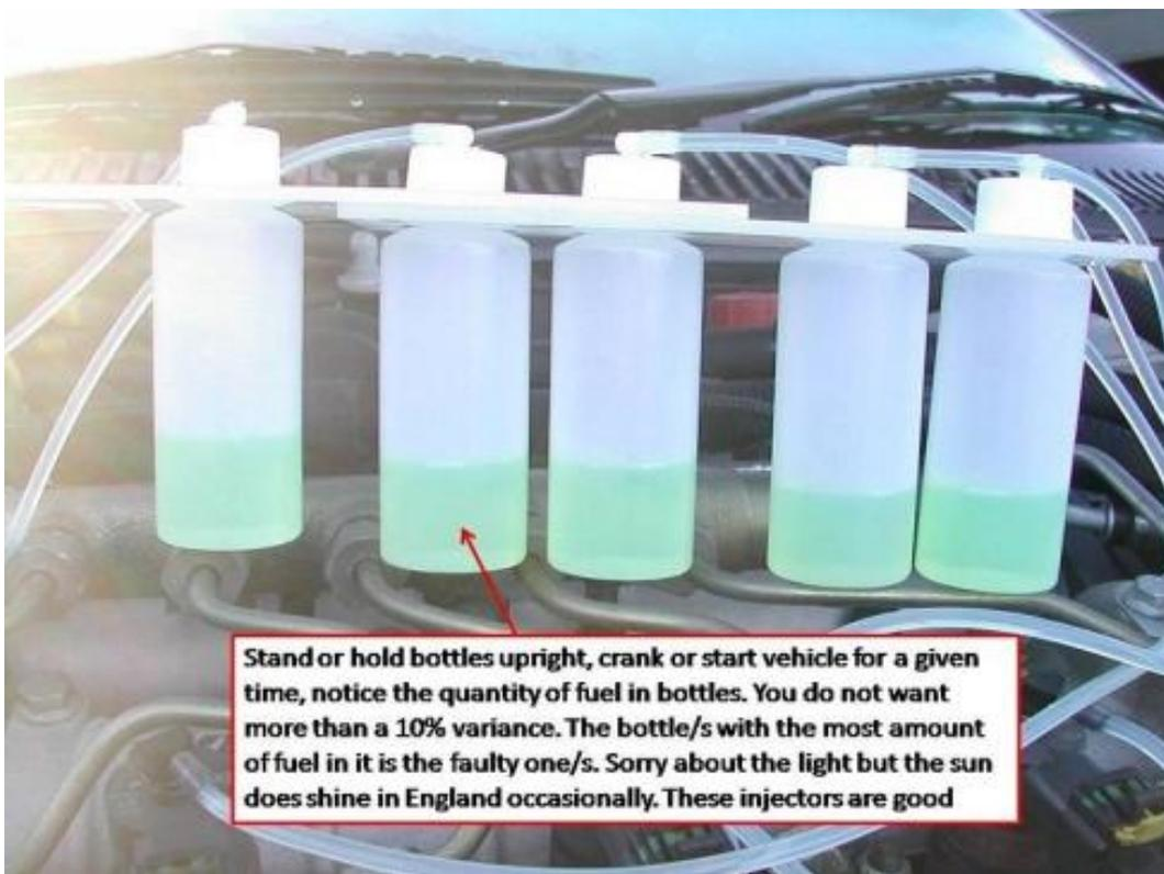
Less than 10% overall variation is ideal. If there is a greater difference between the volumes in the bottles, the injectors delivering more fuel into the bottles will be faulty.
