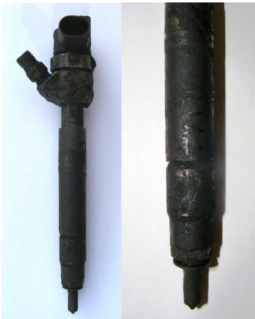
An injector that has suffered from blow-by, notice the carbon up the stem.
