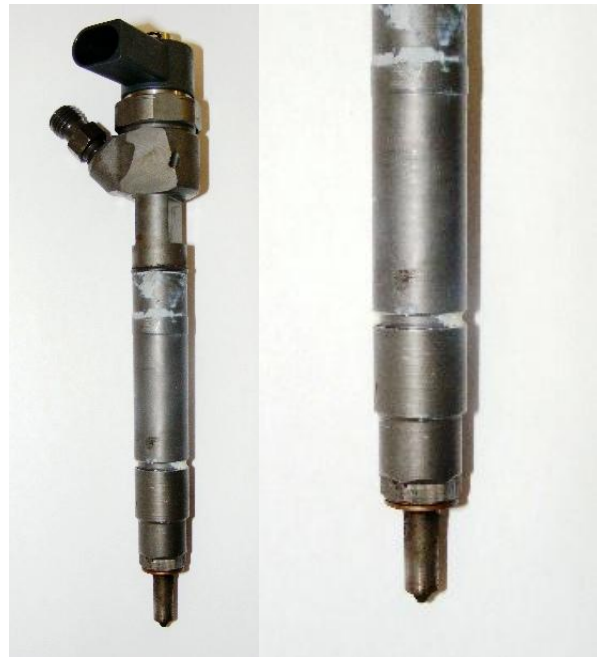
This injector has been seating correctly, the seat and copper washers have prevented any blow-by.
